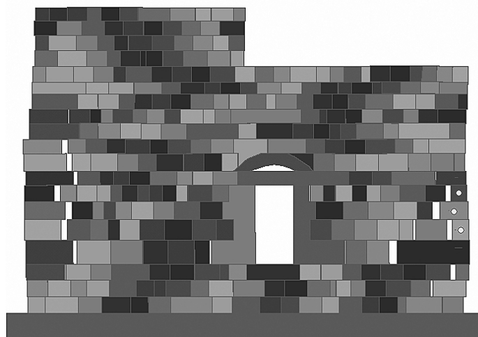
Figure 14. A simulation without a confining wall predicts the exact height of displaced blocks as is observed in the field. A=1.5g , f=5\text{Hz} .
