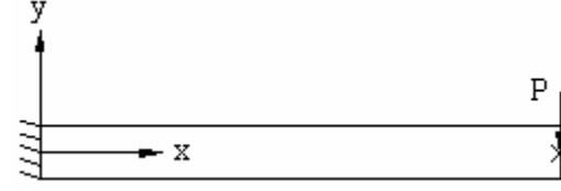
Fig. 4: A cantilever subjected to a vertical force at the mid-point of the free end.
