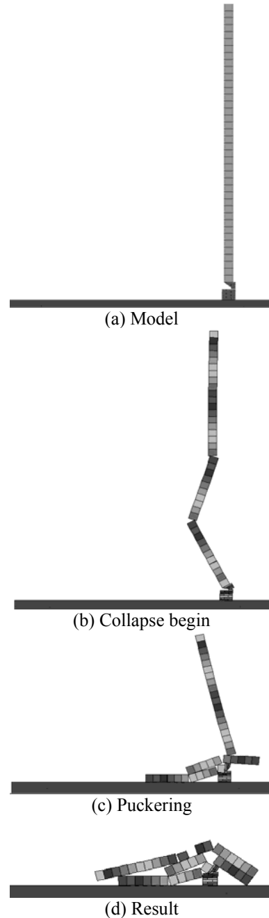
Fig.3: Demolition process of the eastern wall
